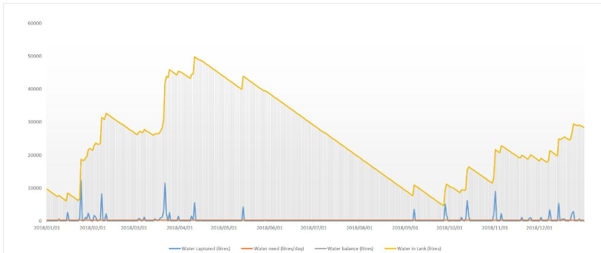
**Figure 7:** Rainwater capture, storage and use over a year with 500 mm annual rainfall, 50,000 L rain tank and 300 m<sup>2</sup> catchment surface.
