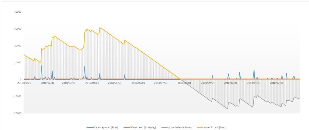
**Figure 5:** Rainwater capture, storage and use over a year with a 500 mm annual rainfall, 40,000 L rain tank and 200 m<sup>2</sup> catchment surface.
