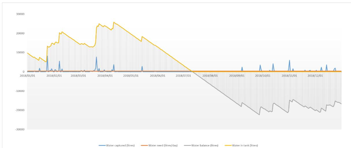
**Figure 6:** Rainwater capture, storage and use over a year with 500 mm annual rainfall, 50,000 L rain tank and 200 m<sup>2</sup> catchment surface.
